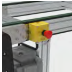
Emergency stop switch Safety option for the immediate stoppage of the conveyor. The emergency stop switch is positioned according to the specific application and integrated into the conveyor line's control system.
